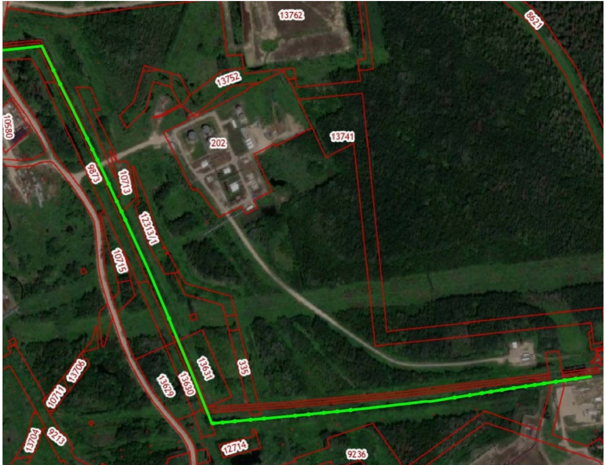
Figure 6 – Fragment of the cable rack route location
